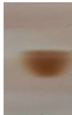
Fraction 1 of ethyl acetate (100%) in developing solvent system methanol: ethyl acetate (5:5). The presence of a brown colored spot indicates the existence of tannins
